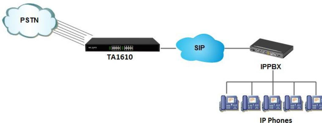
Figure 2-2 Connect IPPBX and TA FXO Gateway
