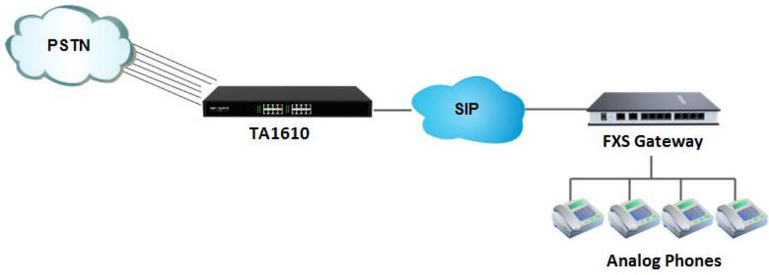
Figure 2-3 Connect TA FXO Gateway and FXS Gateway
